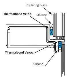
NOTE: Thermalbond V2100 is a SPACER material and not intended to be a structural component.
